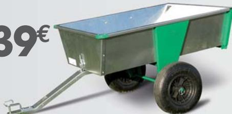
CAISSE TRÈS ROBUSTE EN TÔLE D'ACIER GALVANISÉ D'ÉPAISSEUR 2 MM PLIÉE EN UNE SEULE PIÈCE, PANNEAU AVANT VISSÉ, PANNEAU ARRIÈRE AMOVIBLE PAR COULISSEMENT, FLASQUES LATÉRALES, COINS ARRIÈRE ET ANGLES AVANT POUDRÉS EN COLORIS VERT, TIMON AVANT BASCULANT RELIÉ À LA CAISSE PAR UNE GRENOUILLÈRE, FOURNIE AVEC BROCHE DE FIXATION.
